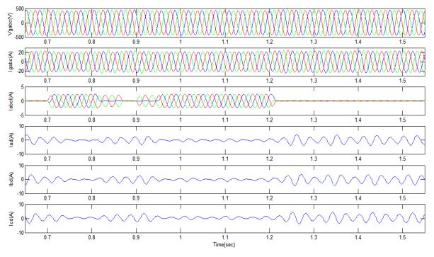
Fig. 2. Simulated transient waveforms of voltage generated by three-phase GIAG ( $V_{gabc}$ ), three-phase GIAG currents ( $I_{gabc}$ ), three-phase resistive load currents ( $I_{abcl}$ ), per-phase DLC currents ( $I_{ad}$ ,  $I_{bd}$ ,  $I_{cd}$ ).
