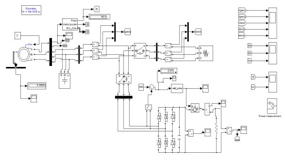
Fig. 1. Simulink model diagram of electronics based DLC
