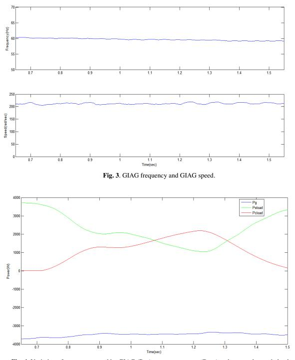
Fig. 4. Variation of power generated by GIAG ( $P_{gen}$ ), consumer power ( $P_{cload}$ ) and electronic load power ( $P_{eload}$ ).
